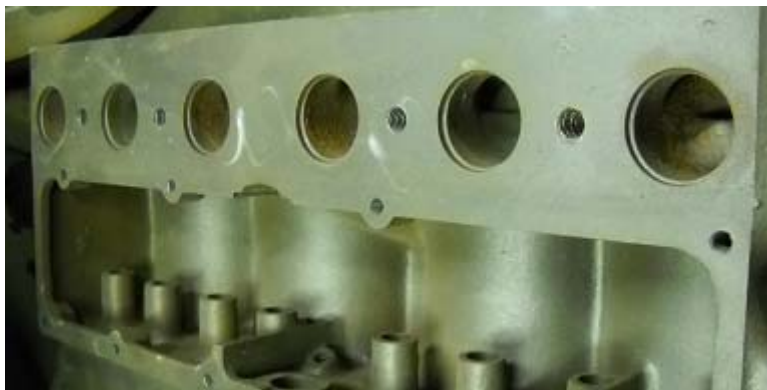
Fig. 26: All Counterbored Ports
