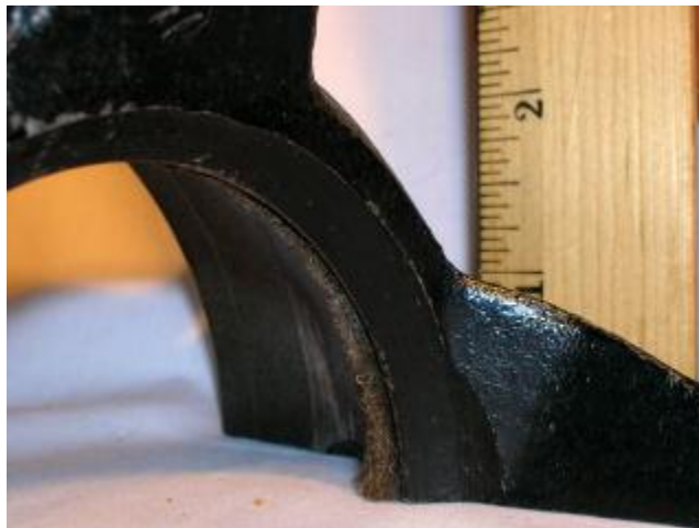
PICTURE OF RIB HEIGHT Universal joint housing—outer lower rib height of 1-1/16 inch.
